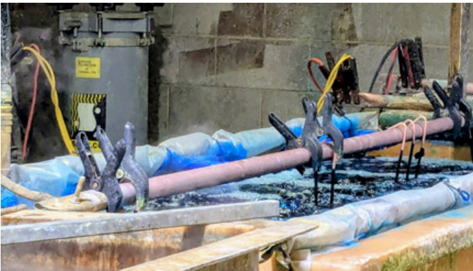
Restoration begins by chemically stripping the old plating down to its original metal.
