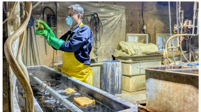
Metals are cleaned in caustic chemical baths to ensure all oils and impurities are removed. Because of the strong odor, we had only seconds to capture this process.
