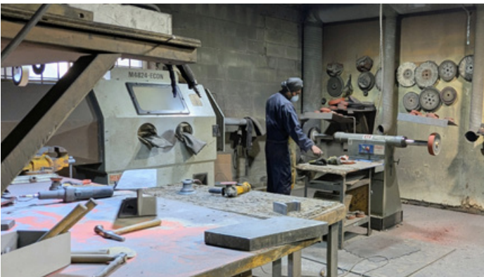
A sandblasting cabinet in the foreground, with work proceeding to remove more rust & paint. The polishing wheels create a look of functional “wall art”.
